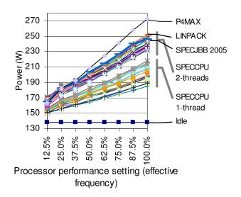
Figure 2: Maximum system-level power measurement for each processor performance state.
