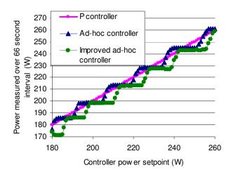
Figure 8: Steady-state error. P4MAX, is run with set points from 180 W to 260 W. The maximum power for a 66 second interval is recorded and the average of 3 runs is plotted. The P controller matched the set point to 0.1 W precision. The ad-hoc controller showed long-term, steady-state violations of up to 6.1 W. The improved ad-hoc controller is run with a safety margin by subtracting 6.1 W from the set point and exhibits no power budget violation.
