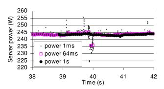
Figure 6: LINPACK without power management. Graph shows 4 seconds of the LINPACK benchmark after running for 38 seconds. Average power over 1 ms, 64 ms, and 1 s periods is plotted. LINPACK has almost constant power consumption with periodic dips in power (as seen around the 40 second mark).
