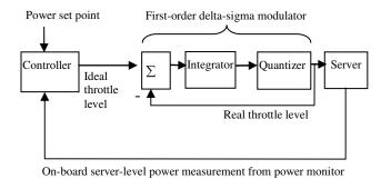
Figure 3: System diagram for power control
