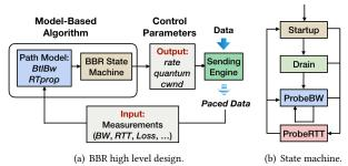
Figure 1: BBR congestion control algorithm design.
