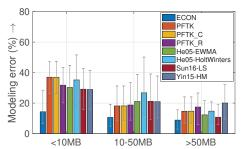
Figure 8: Latency prediction error for different data size ranges. ECON provides greater benefits for smaller data sizes.
