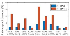
Figure 10: HTTP/1.1 and HTTP/2 latency modeling error for different file sizes and loss rates. For the first three sets of bars, the transfers complete within the TCP slow start phase.
