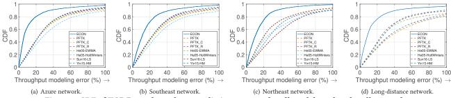
Figure 6: CDF of TCP Reno throughput prediction error under all models and under all networks.
