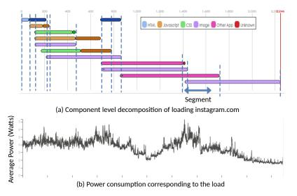
Fig. 2. (a) Using WProf-M to decompose the components when loading the instagram. com Web page. (b) The instantaneous aggregate power draw recorded as the Web page loads. Segments are shown in dashed lines.
