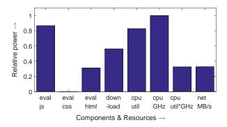
Fig. 11. Normalized power contribution estimations for components and resources based on our LR modeling.
