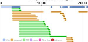
Fig. 13. Illustrating the increased delay in decompressing css (green bars) and js (brown bars) under compression level 9 (bottom) when compared to level 1 (top) for irs.gov.
