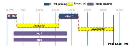
Fig. 1. An example page load process decomposed into various components such as HTML parsing, JavaScript, etc.
