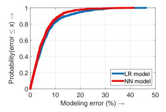
Fig. 6. *RECON* error CDF: The CDF shows the LR and NN energy estimation errors across all runs of all Web pages (800 data points). 83% of the LR errors and 86% of the NN errors are below 10%.
