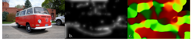
Figure 1. a. The original image; b. The edge confidence map Q (right) extracted from the original image. Brighter pixels indicate higher confidence; c. The gradient directions after smoothing (used to penalize the expected shadow gradient). The x and y components of the gradient are encoded in the red and green channels.
