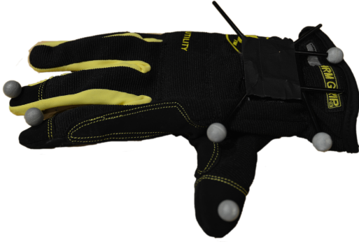
Figure 1: One of the low-cost, passively tracked gloves that we used with our interface. It is constructed by attaching a standard tracking system rigid body to the back of a soft glove, using wires running through the fabric to preserve its elasticity and ensure a deformation-resistant connection. Retroreflective markers are attached on the tips of the thumb, index and middle fingers. The total cost of materials for one glove is under $25.
