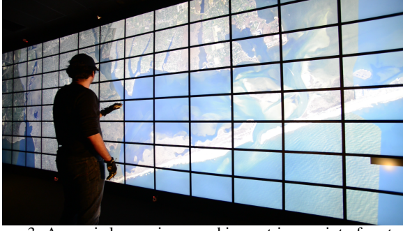
Figure 3: A user is leveraging our chirocentric user interface to explore a 2D GIS dataset on large immersive tiled display wall. The user has just performed a constrained direct-manipulative translation on the 2D map plane.
