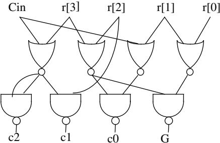
The structure for a carry-with-less-delay organization using 5 such CLA modules is as follows:
