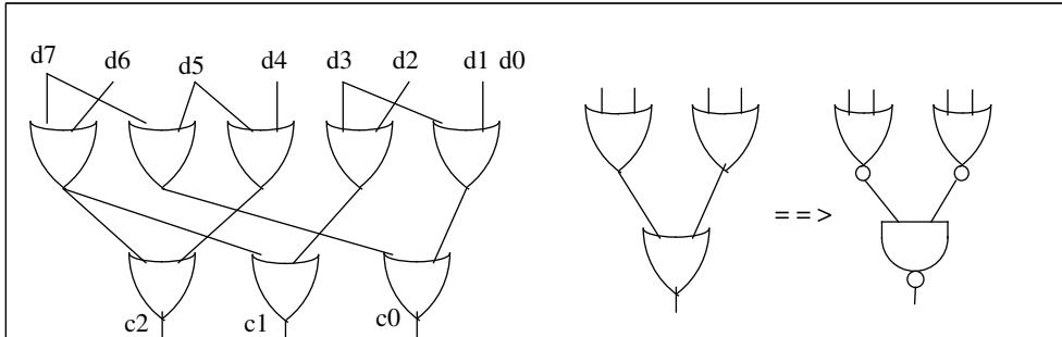
The circuit above is usually derived from the truth table below left via classical methods for the minimization of a multi-output function although in this simple case it can be eyeballed d7: 1 1 1 and then transformed to a net d6: 1 1 0 of NAND/NOR gates d5: 1 0 1 using the equivalence shown d4: 1 0 0 at upper right. d3: 0 1 1 In this case, the synthesizer d2: 0 1 0 could not do better. d1: 0 0 1 (That's what everybody thinks) d0: 0 0 0
