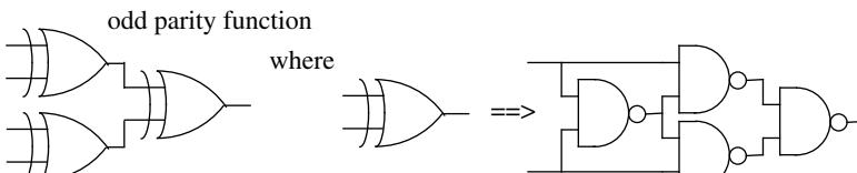
We could reduce the delay from 6 to 5 by also computing the complements of the 2 input exor functions in the first layer, using the circuit on the right, and then combining the four outputs using a tree of three AND gates (but this increases the gate count to 19)
