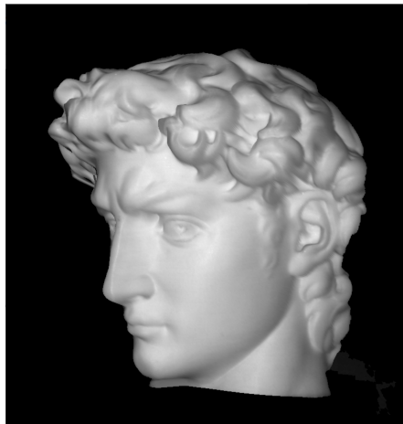
Figure: phase unwrapping mistake.
