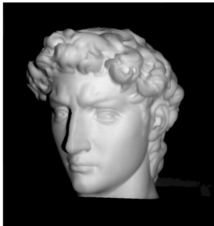
Figure: phase unwrapping mistake.
