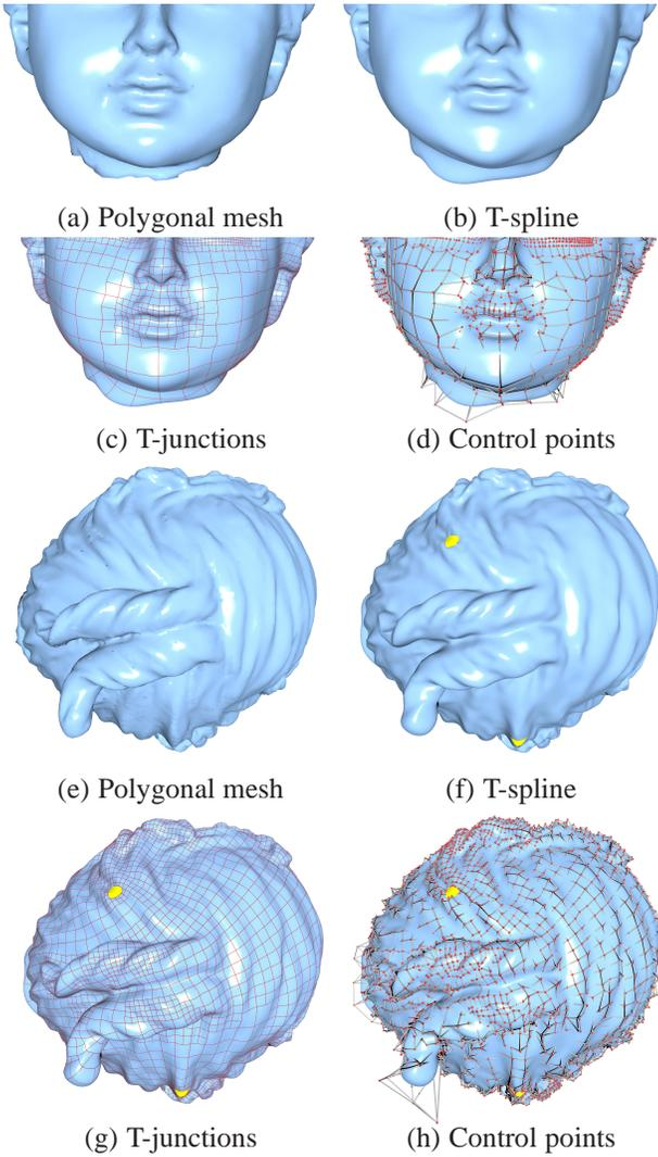
Fig. 9. Close-up views of the reconstructed details. Our hierarchical surface reconstruction algorithm can faithfully reconstruct the details in the original model. (a) and (e) show the original polygonal model. (b) and (f) show the T-spline surfaces of  $C^2$  continuity. (c) and (g) highlight the T-junctions on the spline surfaces. (d) and (h) show the splines overlaid by the control points.
