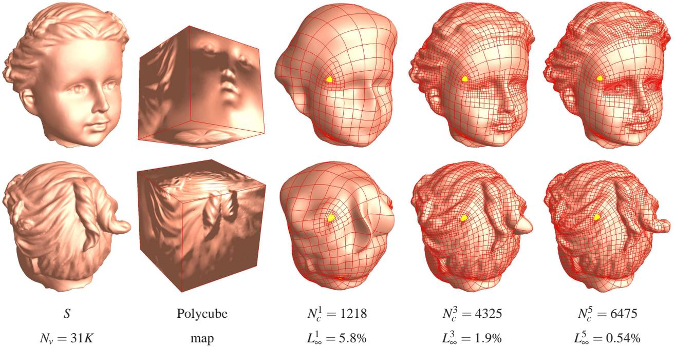
Fig. 8. Hierarchical surface reconstruction of Polycube T-splines.  $N_c^i$  and  $L_\infty^i$  are the number of control points and maximal fitting error in iteration  $i$ .  $N_v$  is the number vertices in the input polygonal mesh  $S$ . The input data is normalized to a unit cube.
