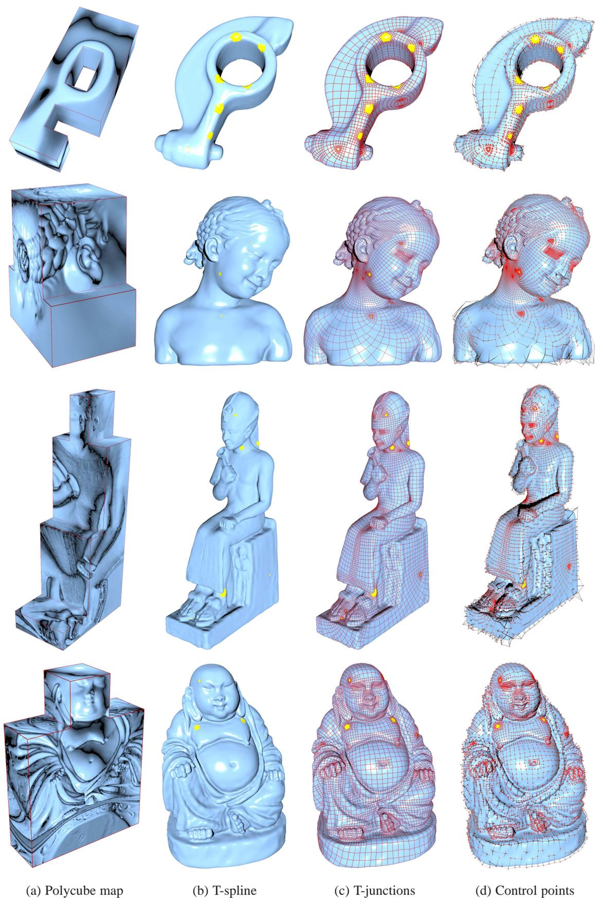
Fig. 14. Construction of manifold T-splines using polycube maps.
