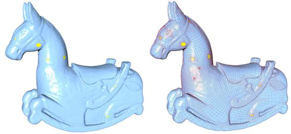
Fig. 11. Polycube T-splines for the Isodore Horse model.
