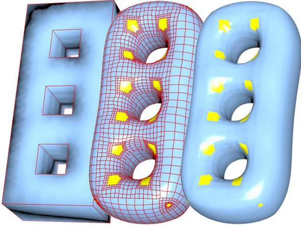
Fig. 1. T-splines on polycubes. The polycube serves as the parametric domain which mimics the geometry of the 3D model. All the corners are singularities which are colored in yellow.
