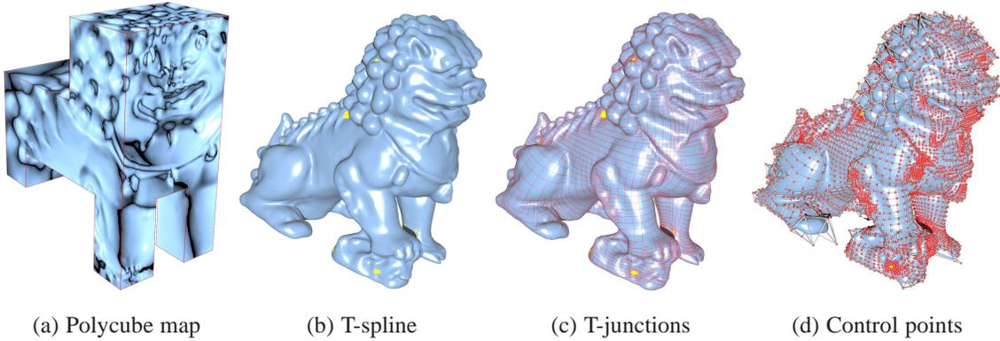
Fig. 12. Polycube T-splines for the Chinese Dragon model.
