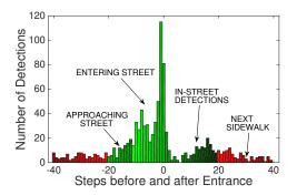
Figure 1: Performance of Crossing Detection Algorithm (Manhattan testbed).
