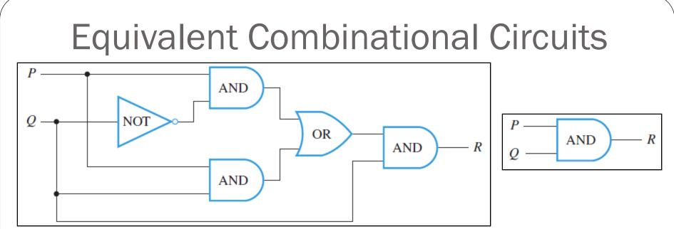
Two digital logic circuits are equivalent if, and only if, their input/output tables are identical.
