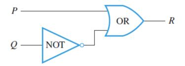
• List the four possible combinations of input signals, and find the output for each by tracing through the circuit.
