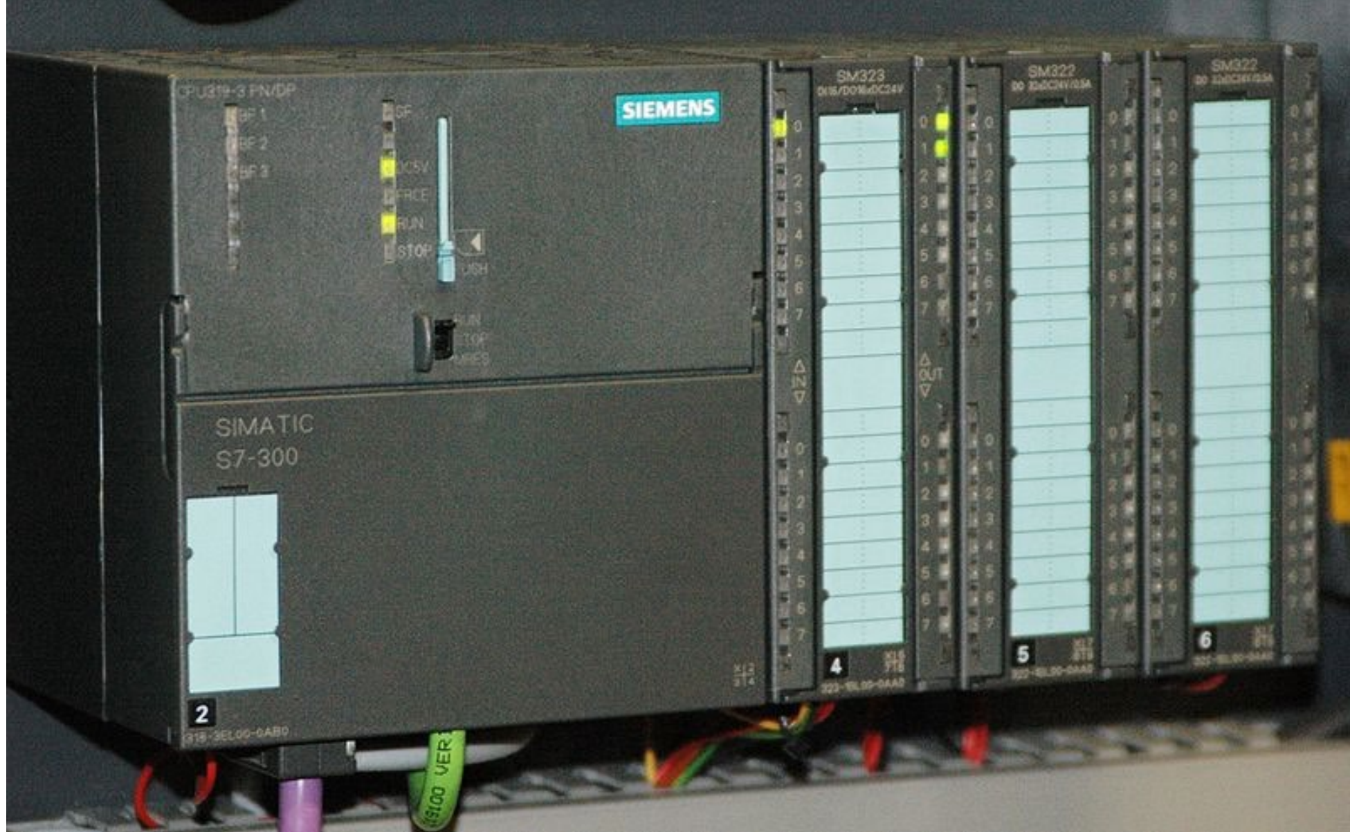
Siemens Simatic S7-300 PLC CPU with three I/O modules attached
