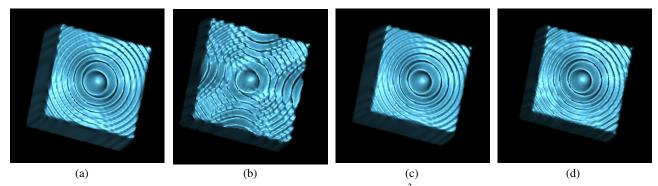
Figure 3: Rendering of the Marschner-Lobb test function on different grids: (a)  $40^3$  CC grid, non-spherical frequency spectrum; (b) BCC grid equivalent to the  $40^3$  CC grid, non-spherical frequency spectrum; (c)  $40^3$  CC grid, constrained to a spherical frequency spectrum; (d) BCC grid equivalent to the  $40^3$  CC grid, constrained to a spherical frequency spectrum.
