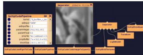
(a) Output data from the pipeline engine is used to create OpenGL textures.
