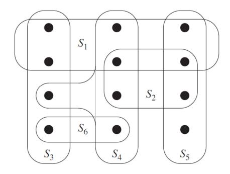
An instance (X, F) of the set-covering problem, where X consists of the 12 black points and  $F = \{S_1, S_2, S_3, S_4, S_5, S_6\}$ . A minimum-size set cover is  $C = \{S_3, S_4, S_5\}$  with size 3. The greedy algorithm produces a cover of size 4 by selecting either the sets  $S_1, S_4, S_5$ , and  $S_6$ , in order.
