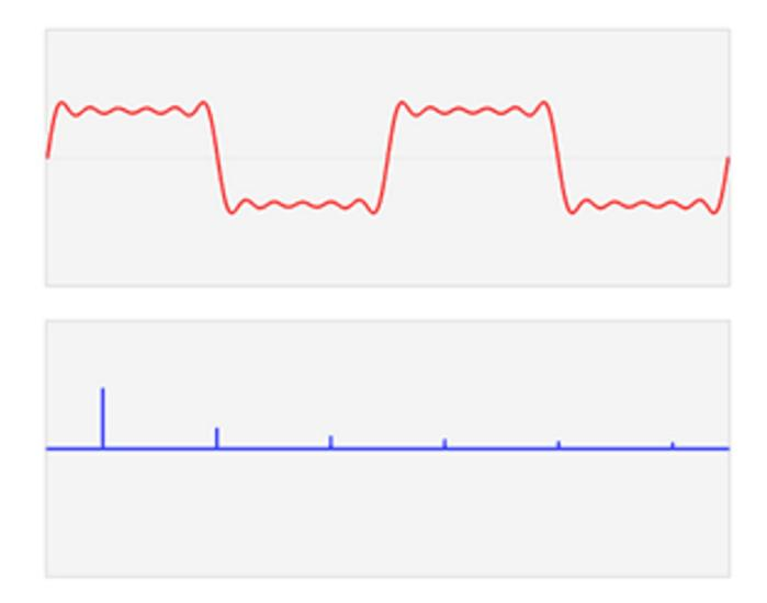
Function s(x) (in red) is a sum of six sine functions of different amplitudes and harmonically related frequencies. The Fourier transform, S(f) (in blue), which depicts amplitude vs frequency, reveals the 6 frequencies and their amplitudes.
