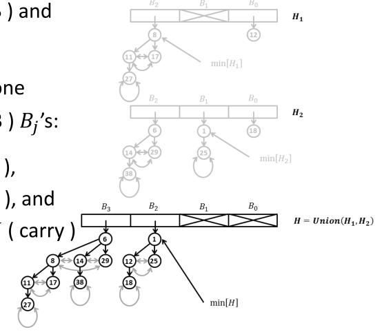
UNION $(H_1, H_2)$  works in exactly the same way as binary addition.
