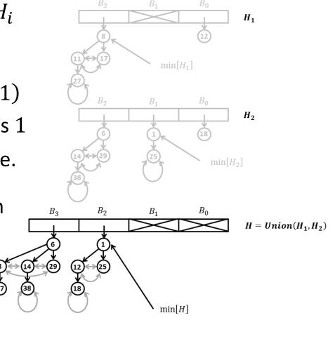
UNION $(H_1, H_2)$  works in exactly the same way as binary addition.
