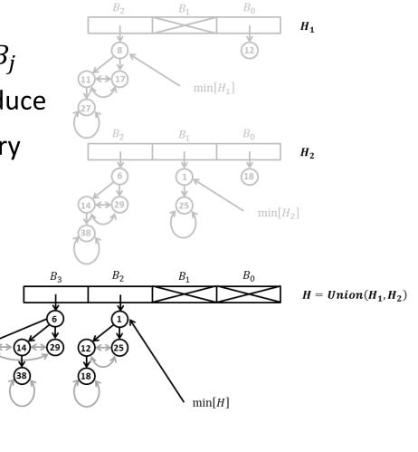
UNION $(H_1, H_2)$  works in exactly the same way as binary addition.
