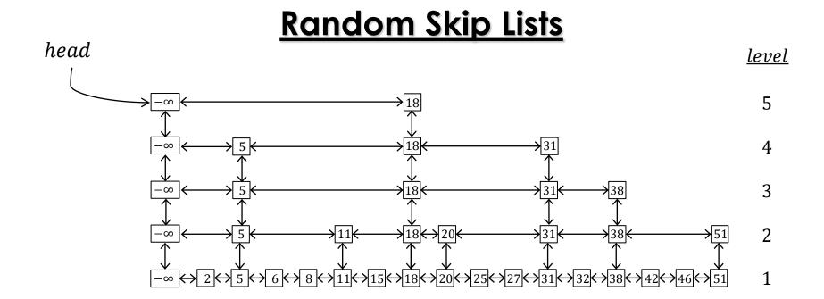
Clearly, for each  $x \in L$  and  $k \ge 1$ ,  $\Pr[l(x) = k] = \frac{1}{2^k}$ . Then  $\Pr[l(x) > k] = \sum_{i=k+1}^{\infty} \Pr[l(x) = i] = \sum_{i=k+1}^{\infty} \left(\frac{1}{2^i}\right) = \frac{1}{2^k}$ .  $\therefore \Pr[h(L) \le k] = \prod_{x \in L} \Pr[l(x) \le k] = \left(1 - \frac{1}{2^k}\right)^n$ .
