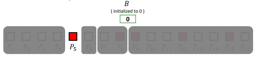
After stage 1: B=1, and so processors  $P_9$ , ...,  $P_{16}$  are eliminated.
