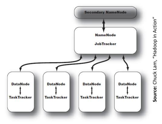
**Secondary NameNode:** It communicates with the NameNode to take periodic snapshots of the HDFS metadata. Does not keep track of any real-time changes to HDFS. Can be configured to work as the NameNode in the event of the failure of the original NameNode.
