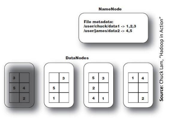
**NameNode:** The bookkeeper of HDFS: keeps track of how files are broken down into file blocks, which nodes store those blocks, and the overall health of the distributed filesystem.
