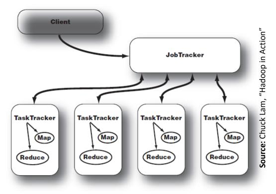
**JobTracker:** Determines the execution plan for a job by determining which files to process, assigns nodes to different tasks, and monitors all tasks as they're running. Should a task fail, the JobTracker will automatically relaunch the task, possibly on a different node.
