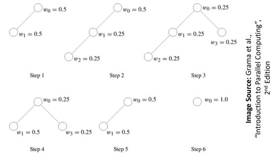
Suppose, initially, only processor 0 has any work. We set  $w_0 = 1$ , and  $w_i = 0$  for i > 0.
