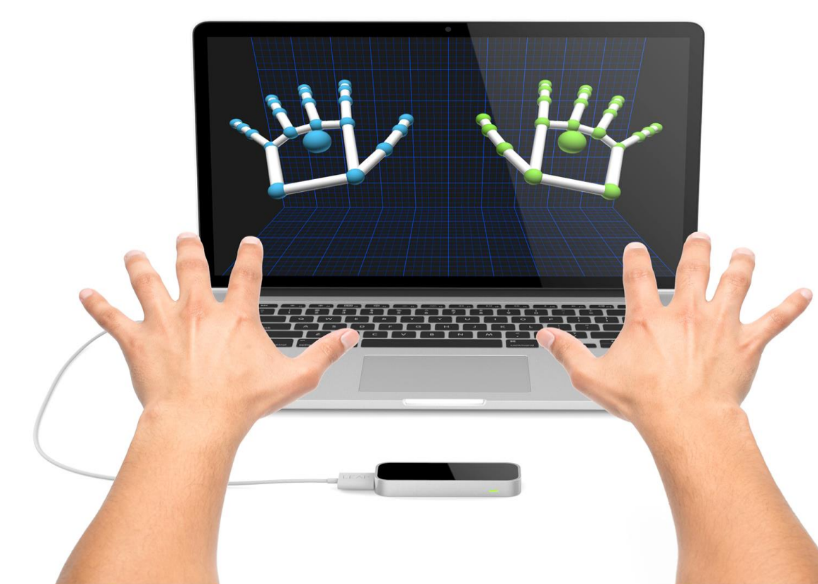
Figure 4: Demonstration of hand tracking using leap motion sensor
