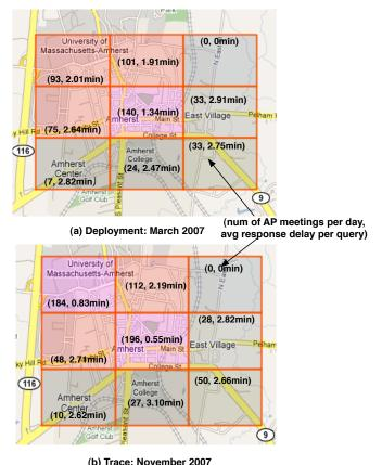
Figure 6: Deployment and Trace: Number of m2i contacts and average delay classified according to geographical locations. The map is a 2 sq.mile snapshot of the DieselNet testbed around Amherst Town center.
