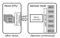
Figure 1. A typical sensor hub architecture.
