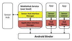
Figure 7. MobileHub implements a sensor hub service at the user level to interface the sensor hub with the application.
