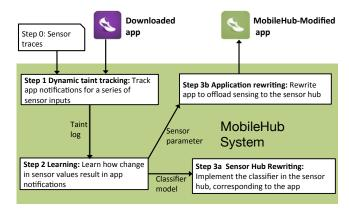
Figure 2. The MobileHub architecture
