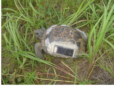
Figure 2.1. Background: A solar-powered tracking device used in TurtleNet.
