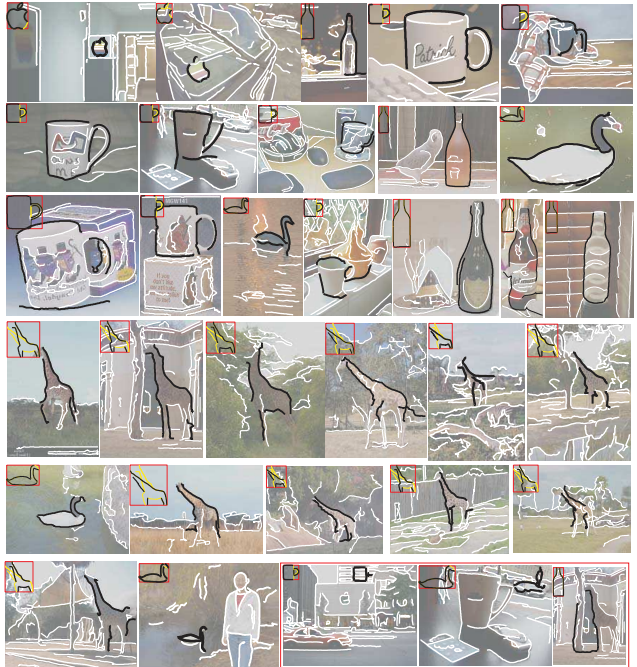
Figure 9. Sample detection results. The edge map is overlaid on the image in white. The detected fragments are shown in black. The corresponding model parts are shown in top-left corners. The red frame in the bottom row shows some false positives.
